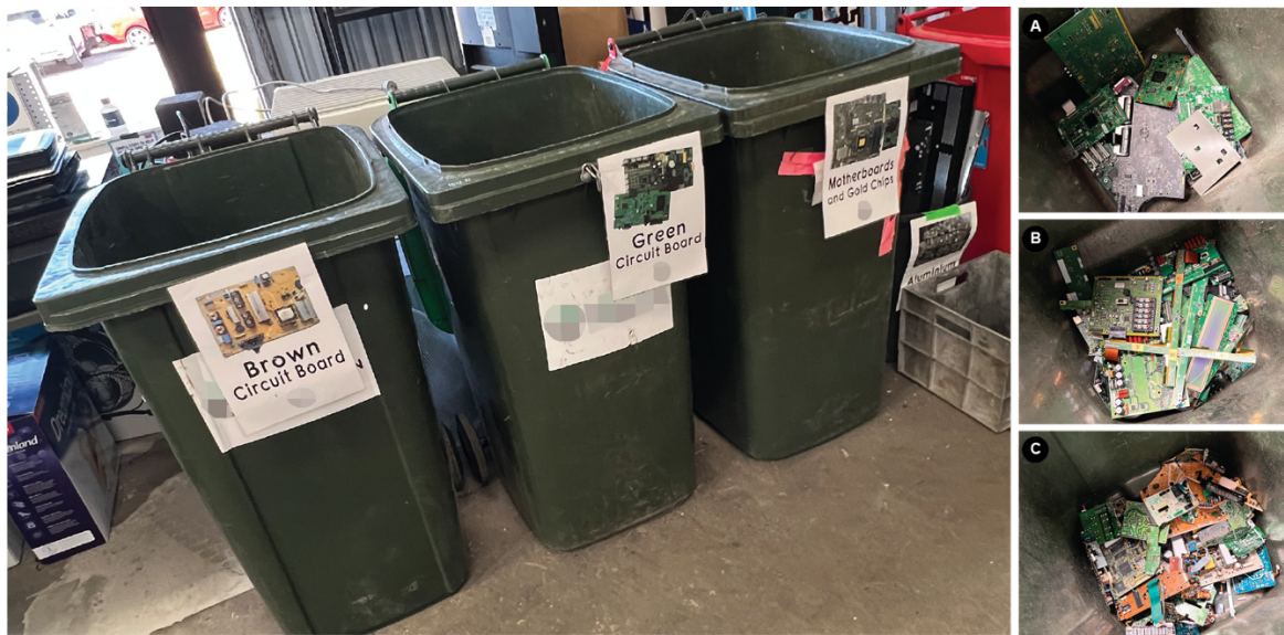
Figure 2: e-Waste recycling social enterprise bins, for people to place components into after disassembling devices, based on the value of their components. (A) motherboards + gold chips; (B) green circuit board; and (C) brown circuit board
